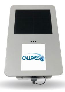
Solar Sense is an energy-harvesting LTE Cat 1 Asset Tracker that supports long-term, remote deployments without the need to replace the battery.
