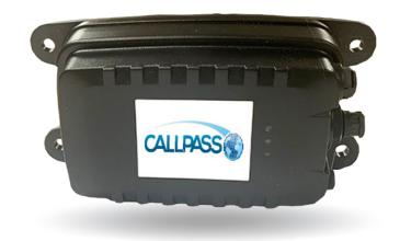
CP47 is a self-contained LTE Cat1 modem with integrated GPS engine, cellular antennas, accelerometer, motion detector, Wi-Fi and Bluetooth for optional wireless sensor integration, and 5 Ah internal rechargeable battery.
